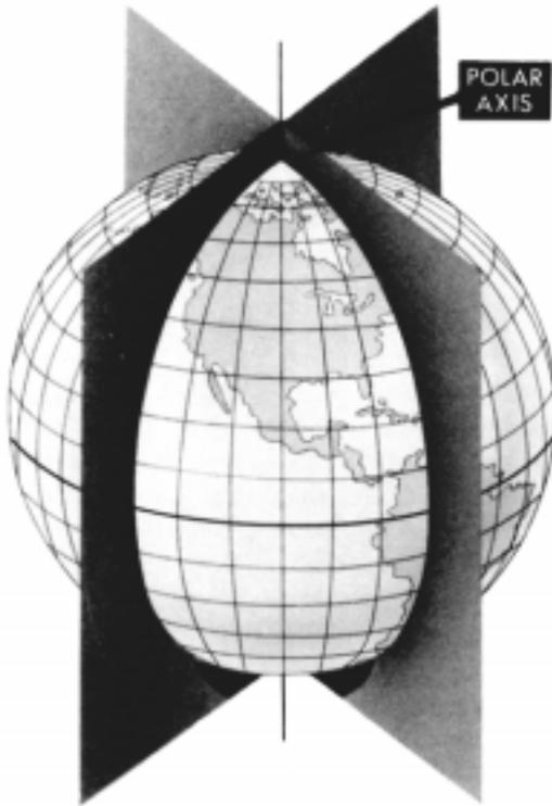
Figure 104a. The planes of the meridians meet at the polar axis.
