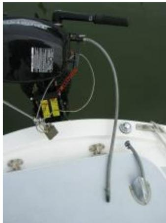
Disconnect the motor from the tank at the coupling by pressing the gray plastic tab and pulling apart the male and female parts of the coupling (see photos below). When connecting the line, press the gray tab and firmly push the male and female parts together so that they are fully engaged, then release the tab. You may need to twist side to side while pushing to get the two ends to fully engage. Tug lightly on the two ends to make sure that they are locked together.
