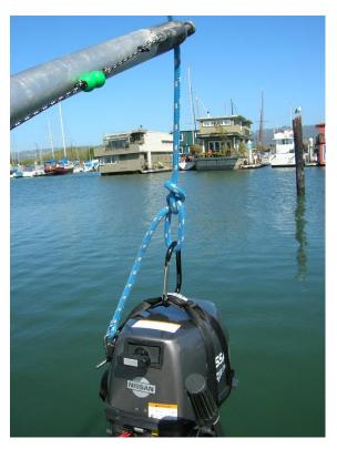
Tie a safety line to the motor and loosen the clamping screws. If removing the motor from the boat, undo the motor security cable and the fuel line.
