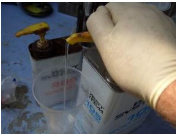
The west systems epoxy pumps deliver the right proportion of resin to hardener, which is critical to a good repair. If the proportion is off, the epoxy won't harden.
