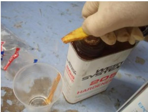
One squirt of resin, and one squirt of hardener provides about two tablespoonsfuls of mixed resin/hardener, which is way more than enough for a ding repair.
