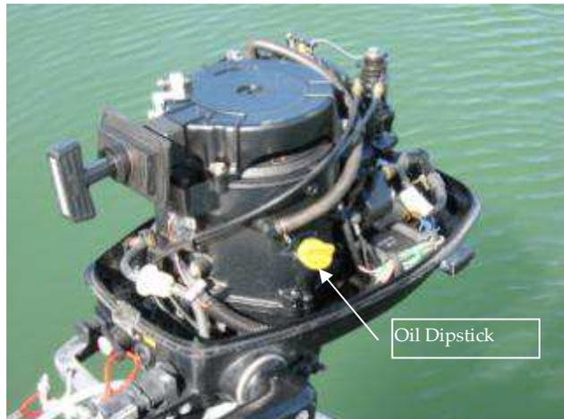
Figure 4 - A Mercury with the engine cover removed
