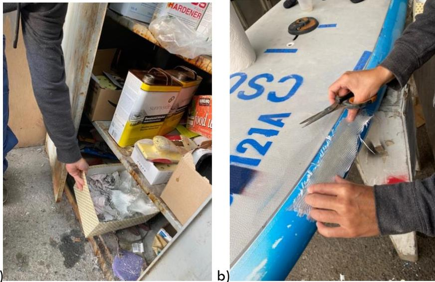
Figure 2. Cutting fiberglass to size. a) the fiberglass box in the locker. b) cutting the fiberglass to make sure it covers the dent and beyond.
