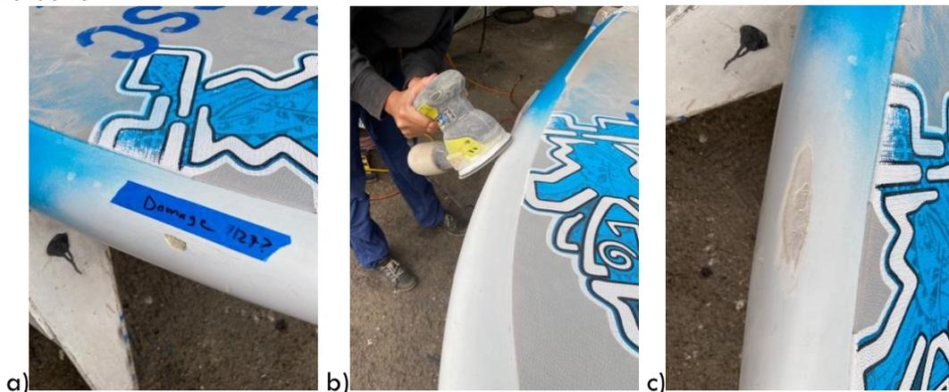
Figure 1. Sanding down a damaged area
