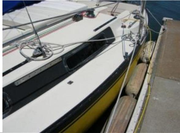
Why: Spring lines help stop the boat from moving forward or backward. The bow and stern lines will still allow the boat to move around unless they are very tight, which they should not be.
