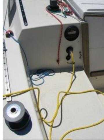
Why: The boat moves around. If the cord is wrapped tightly around something, the boat will put tension on the cord and the fasteners that hold it to the dock.
