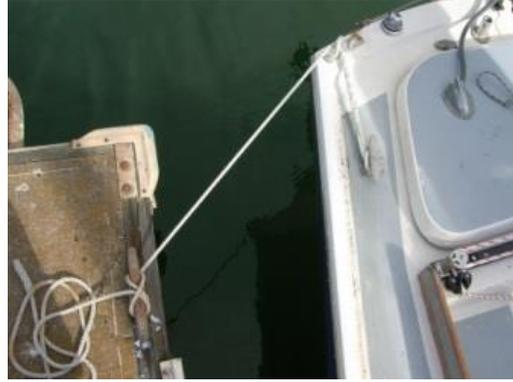
Why: On the Commanders, the aft chocks give the stern lines a better angle to the cleat. Chocks can keep the line from rubbing against the deck, too.
