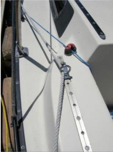
Do: Use the excess bow and stern lines as aft and forward spring lines. They can be tied to the shroud turnbuckles or the winches (or the stanchions, as long as they are tied close to the deck).
