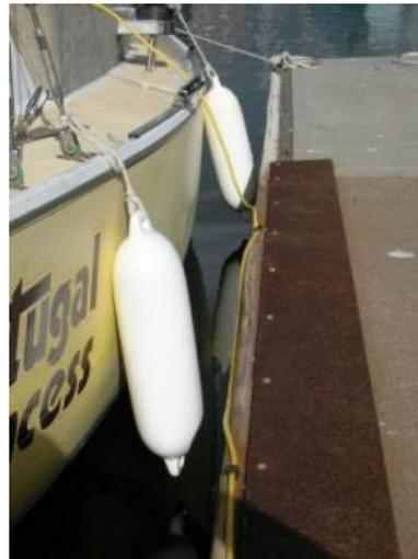
Why: If the fenders are being pinched, that means the dock lines are taut, and the dock lines can wear quickly where they run through the chocks if they are under a lot of tension. In addition, most of our keelboat hulls are painted. If the fenders are squeezed between the dock and the hull, they will wear away the paint on the hull. The fenders will also lose air faster if they are constantly being squeezed.
