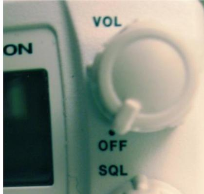
Why: Leaving the radio on will shorten the life of the display. If you forget to plug in the power cord, the radio will run down the battery.
