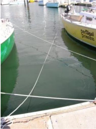
Do: Pull in on the spring line until the bow lines are fairly taut, then ease the spring line a few inches and make it fast. There should be some slack so that the dock lines are not too taut.
