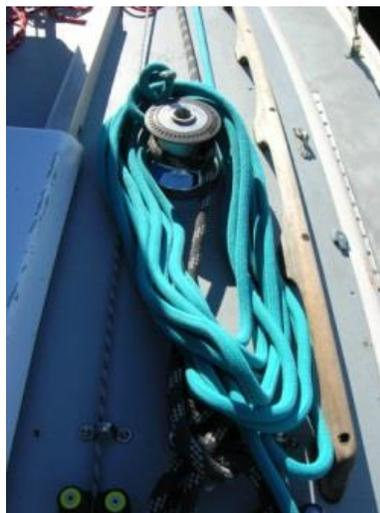
Why: The lines are often wet, especially if you rinse off the boat after sailing, and they tend to stay wet for a long time if they are bunched up. If lines are in close contact with the wood, the wood absorbs water and stays moist, which promotes rot (note the dark spots on the handrail where this halyard was tied).
