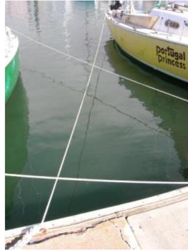
Why: As with fenders, lines hanging in the water quickly attract marine life and become a real mess. A slack spring line may also indicate that the line is not preventing the boat from drifting back.
