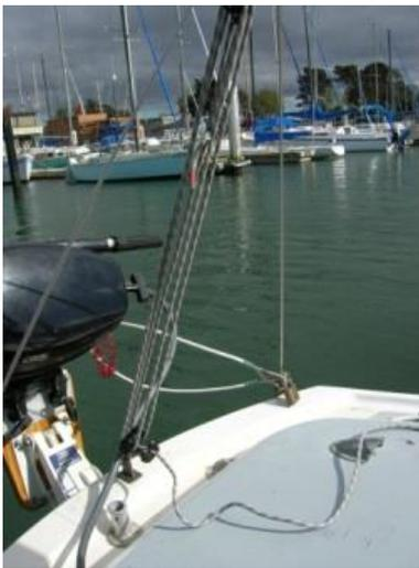
Do: Make sure there is some slack in the backstay tensioner (it should still be cleated, though).
