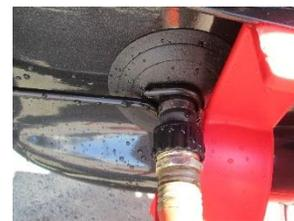
Flushing clears corrosive salt water from the engine. It's only effective if the engine is warmed up enough so that its thermostat is open. Usually you'll drive the skiff to the hoist, hoist it out, and immediately flush it, so the engine will still be warm. If the engine is cold when you start to flush it, you'll need to run it for several minutes to get it warm.
